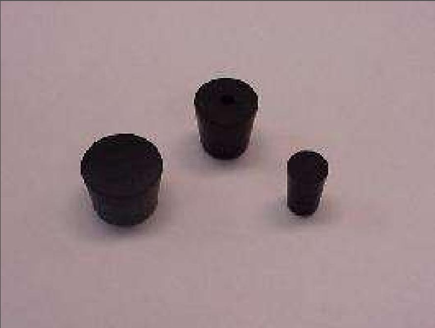
Rubber stoppers are used to close containers to avoid spillage or contamination.
