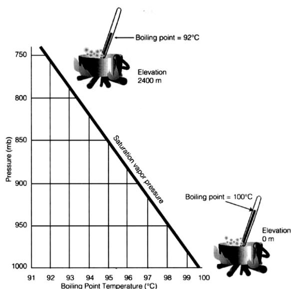
➤ Atop Mount Everest atmospheric pressure is 34 kPa. The vapour pressure of water will reach 34 kPa at about 70°C.
